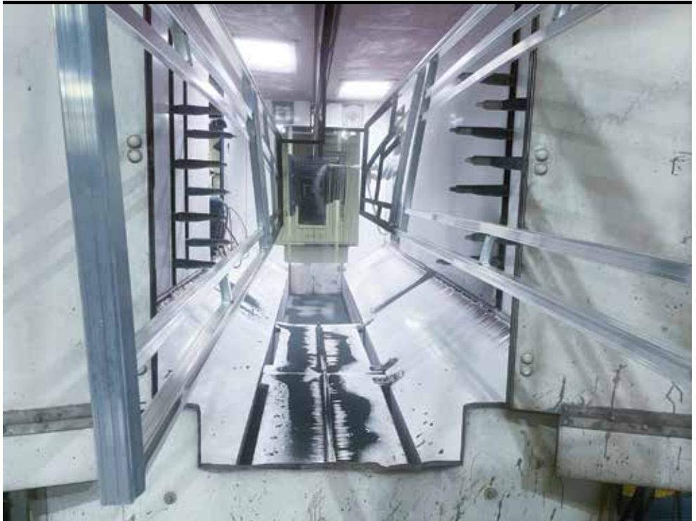
Rails undergoing powder coating process at Winona.
