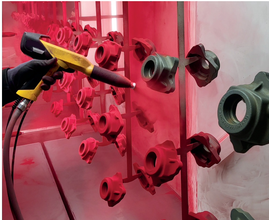
Bearings are powder coated as they are conveyed through the booth.
